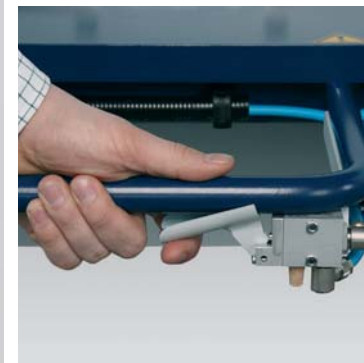
The pneumatic bending support is controlled by a finger lever on the folding beam handle. A pneumatic cylinder assists the operator in bending the piece. You only need compressed air supply.
