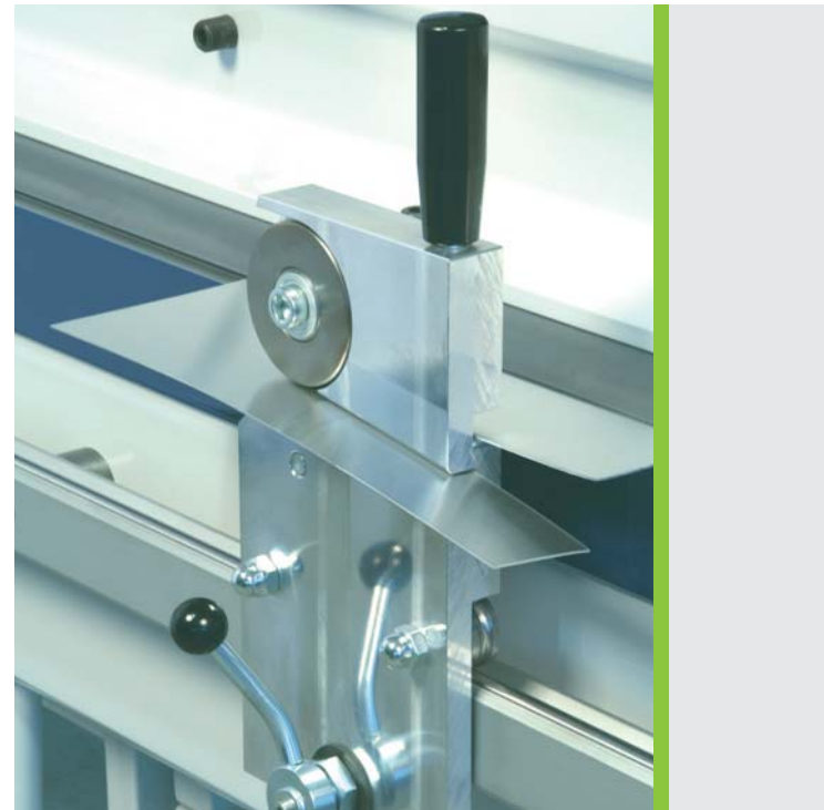
The cutting device is used for safe and easy cutting of ST37 sheets with a material strength of up to 0.8 mm.
