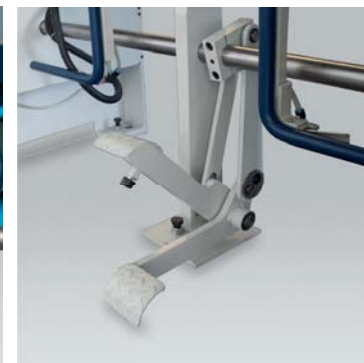
The pneumatic bending support is controlled by a finger lever on the folding beam handle. A pneumatic cylinder assists the operator in bending the piece. You only need compressed air supply.
