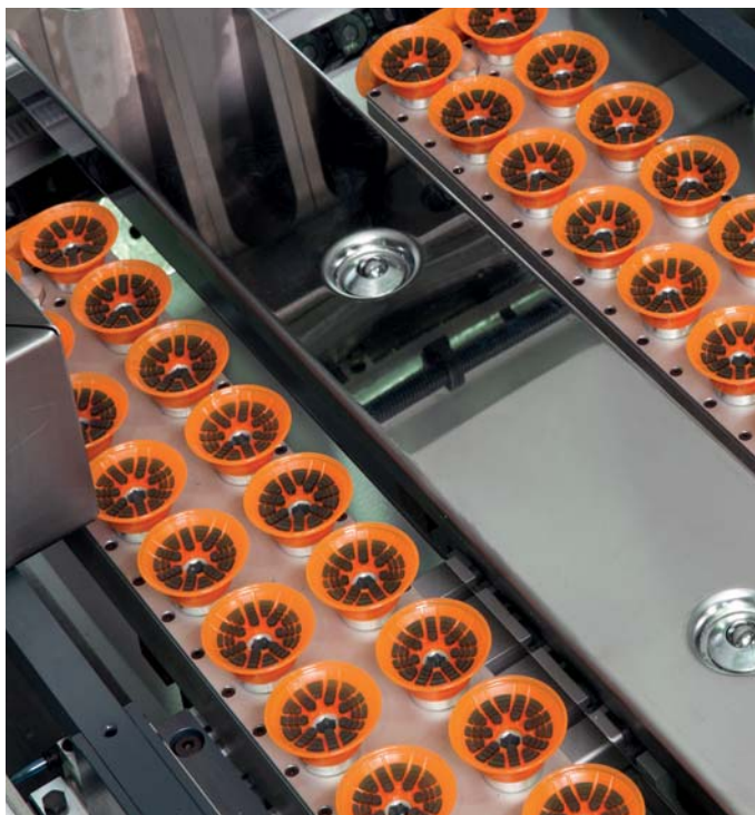
Suction cups in gauge table, controlled via POS 3000.
