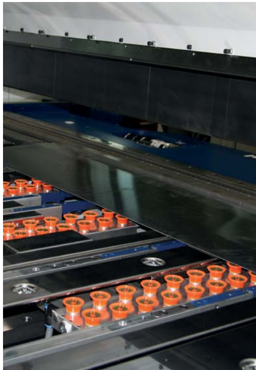
With the optional suction gauge all folds on one side can be done with one simple move by the operator
