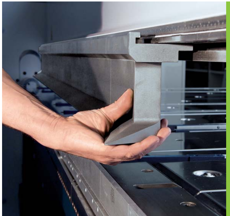
The hydraulic tool clamping device on the clamping beam reduces set-up times.
