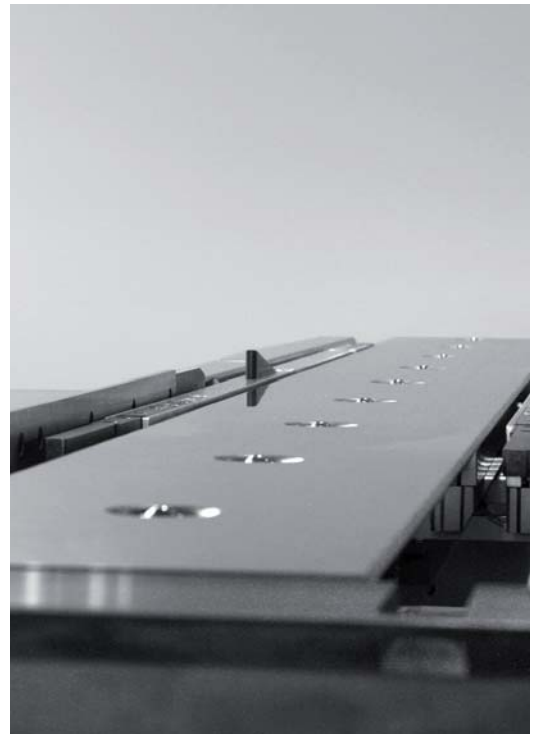
Pneumatic pop up square arms assembled aisle side and gauge fingers ensure a precise positioning of the sheet.
