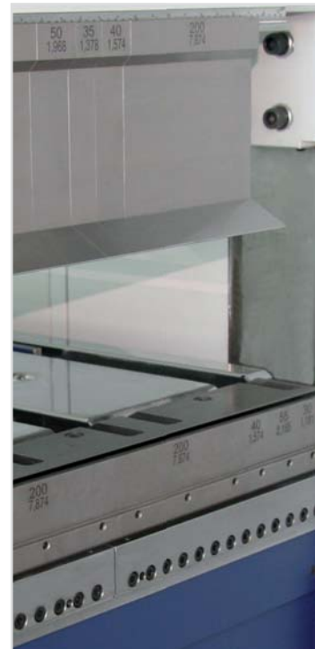
The motor-driven lowerable folding beam and the motorized folding centre adjustment are included in the standard version.
