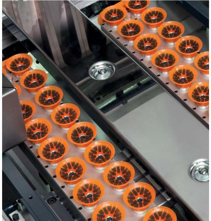
Suction plates in gauge table, controlled via POS 3000.
