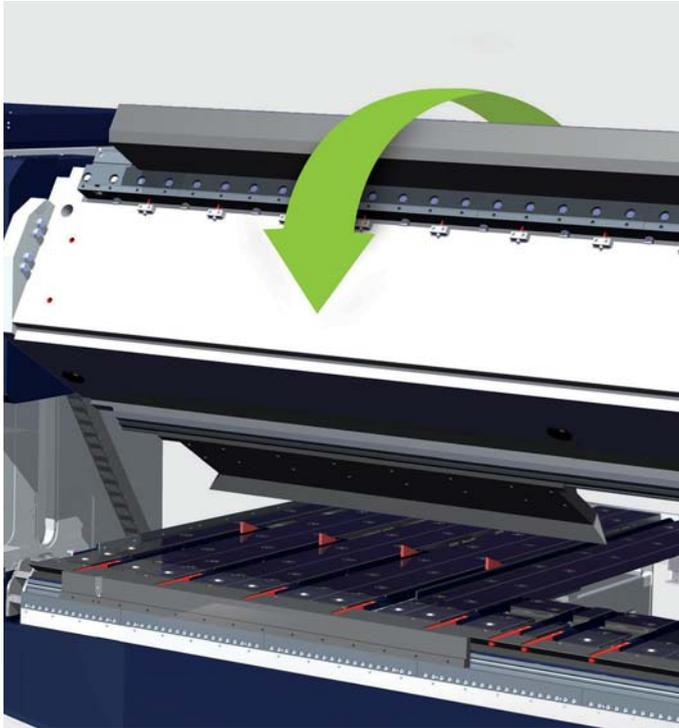
The rotating clamping beam holds a second set of tools.
