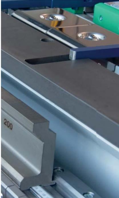
Bottom beam blade with finger grooves
