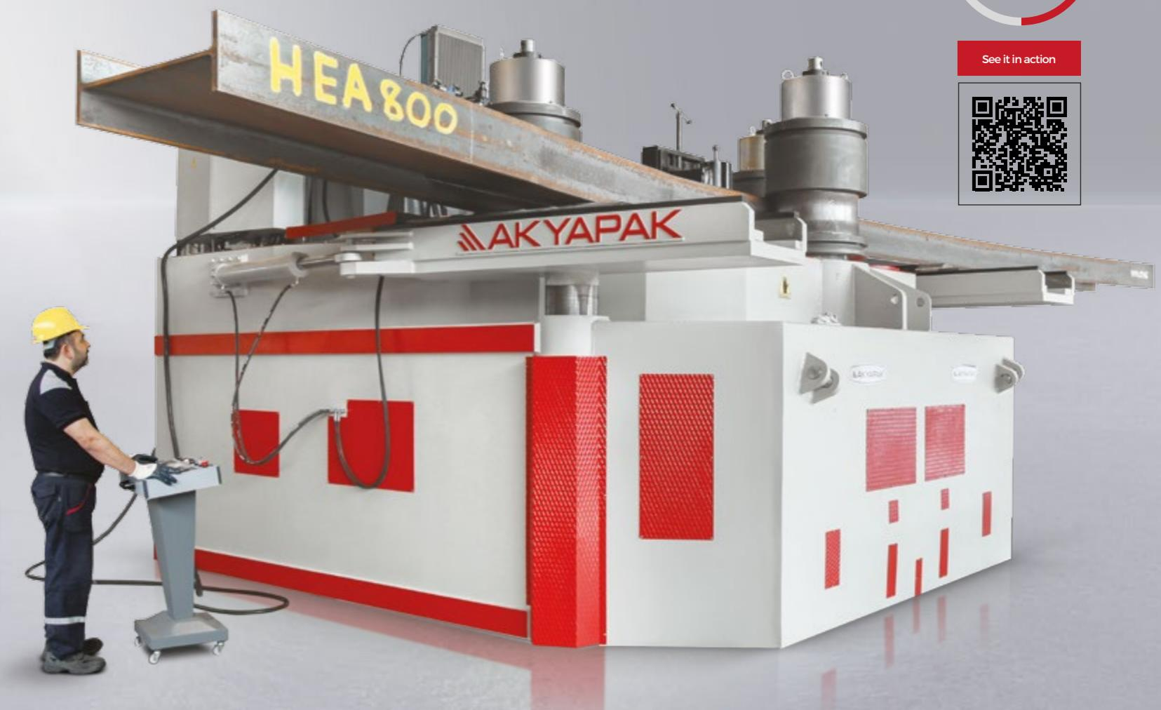
**AKYAPAK offers extensive alternatives on heavy duty profile bending machines as well. Our machines are strong and reliable with their St-52 weld construction body. Minimum flexion causes less deformation, by the help of our machines' enlarged roll diameters. By the help of big measurements of bearings, durability and high bending momentum can be obtained.**
