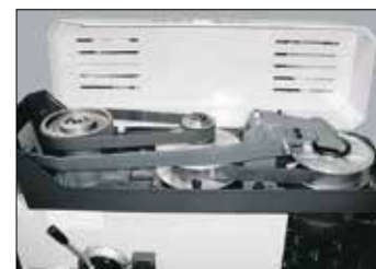
VS: Variable speed-drive unit.
