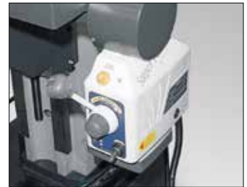
Cod. 40026 Power: Mechanical longitudinal cross-table feed.
